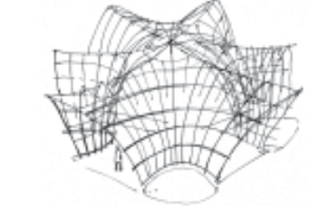
Construction principle of the Visitors' Centre
