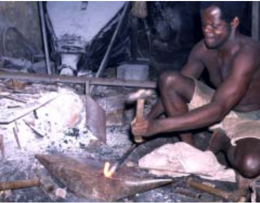
A blacksmith bending iron anchors for the Visitors' Centre
