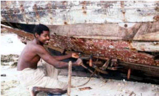
The repetition of the 'dhau' falling dry on the rocky tidal flat on Chumbe Island made boat repairs neccessary. These were carried out by local ship builders.
