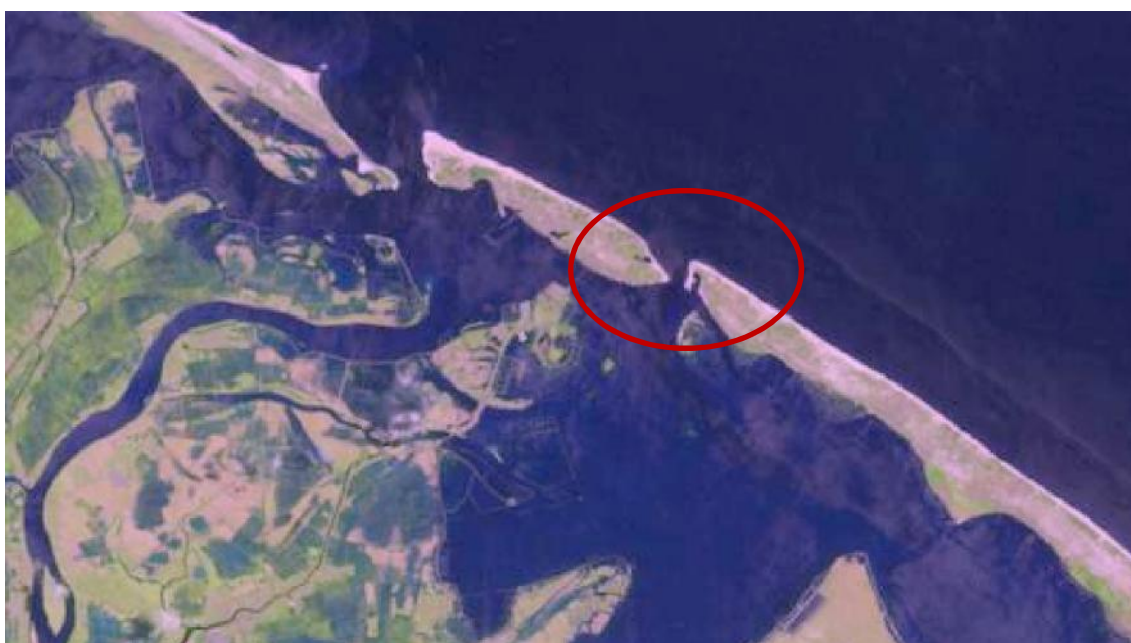
Figure 1: Breach in sand dune near Hue city in 2001 after tropical storm Eve
