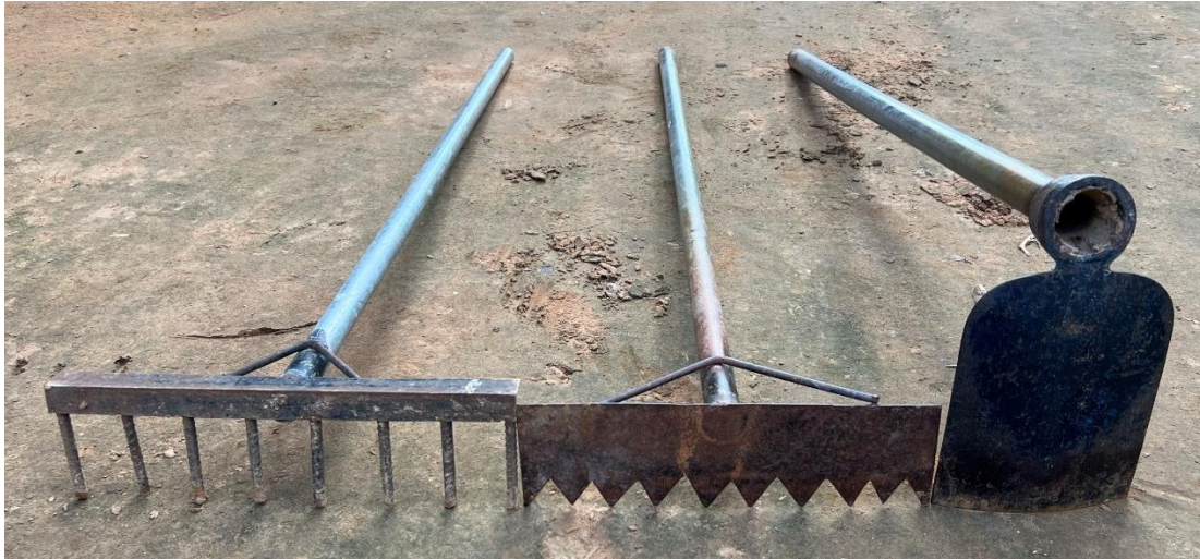
Hand tools for clearing vegetation
