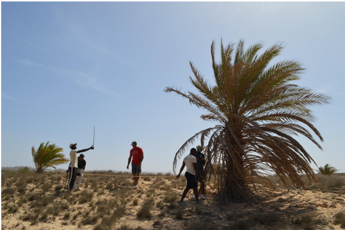
Figure 12: Height measurement of a P. atlantica individual with the proportion technique of Talete's theorem.
