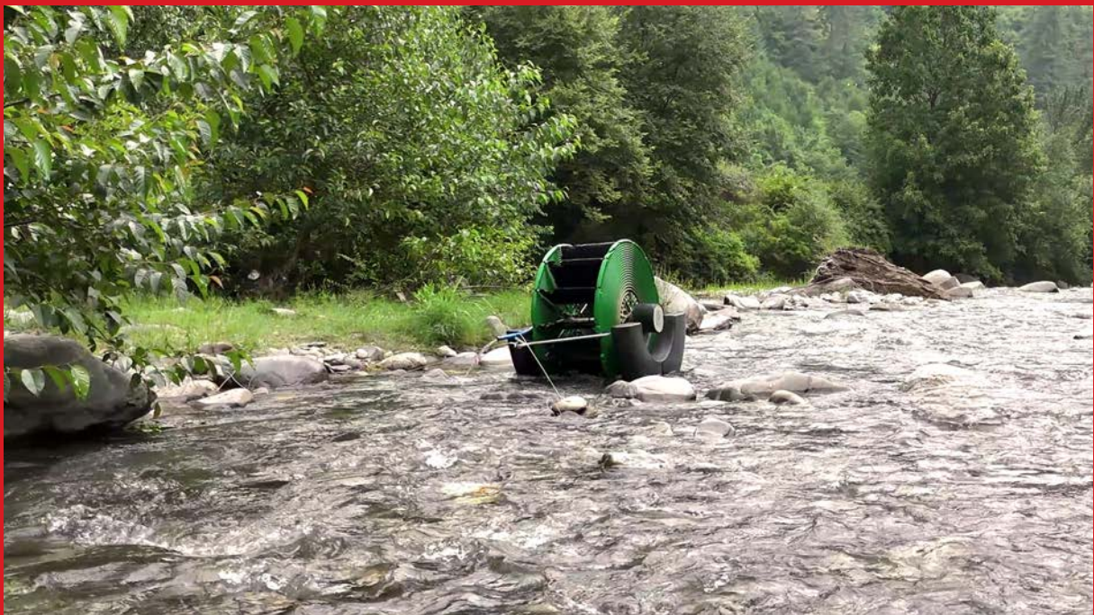
A hydro-powered water pump, installed in 2021 in Gumma village in Shimla, is serving multiple farmers for their irrigation needs.
