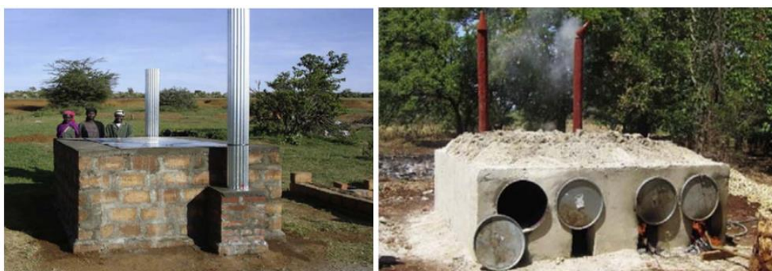
Figure 4. Left : Adam retort kiln, Right : Drum retort kiln
