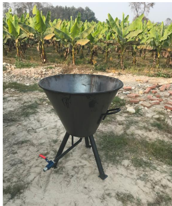
Figure 28. Metal Kon-Tiki kiln design (left) and actual kiln (right)
