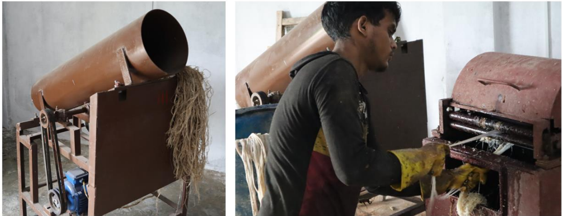
Figure 22. Trunk cutter (left) and banana fibre extraction (right)
