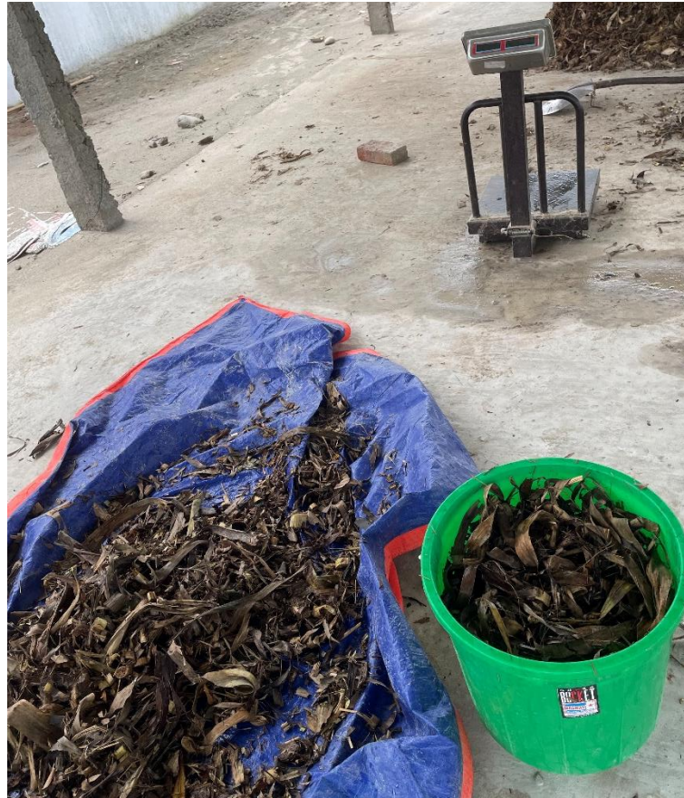
Figure 51. Bulk density and FAS measurements at the fibre factory.
