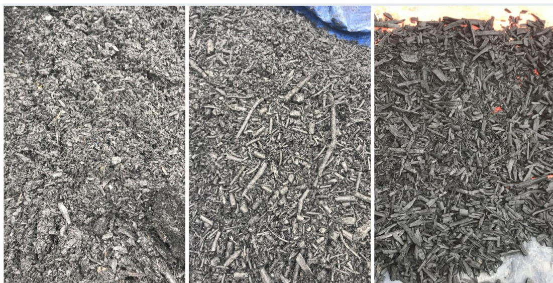
Figure 41. Produced biochar: banana leaves (left), lantana (middle), bamboo (right)
