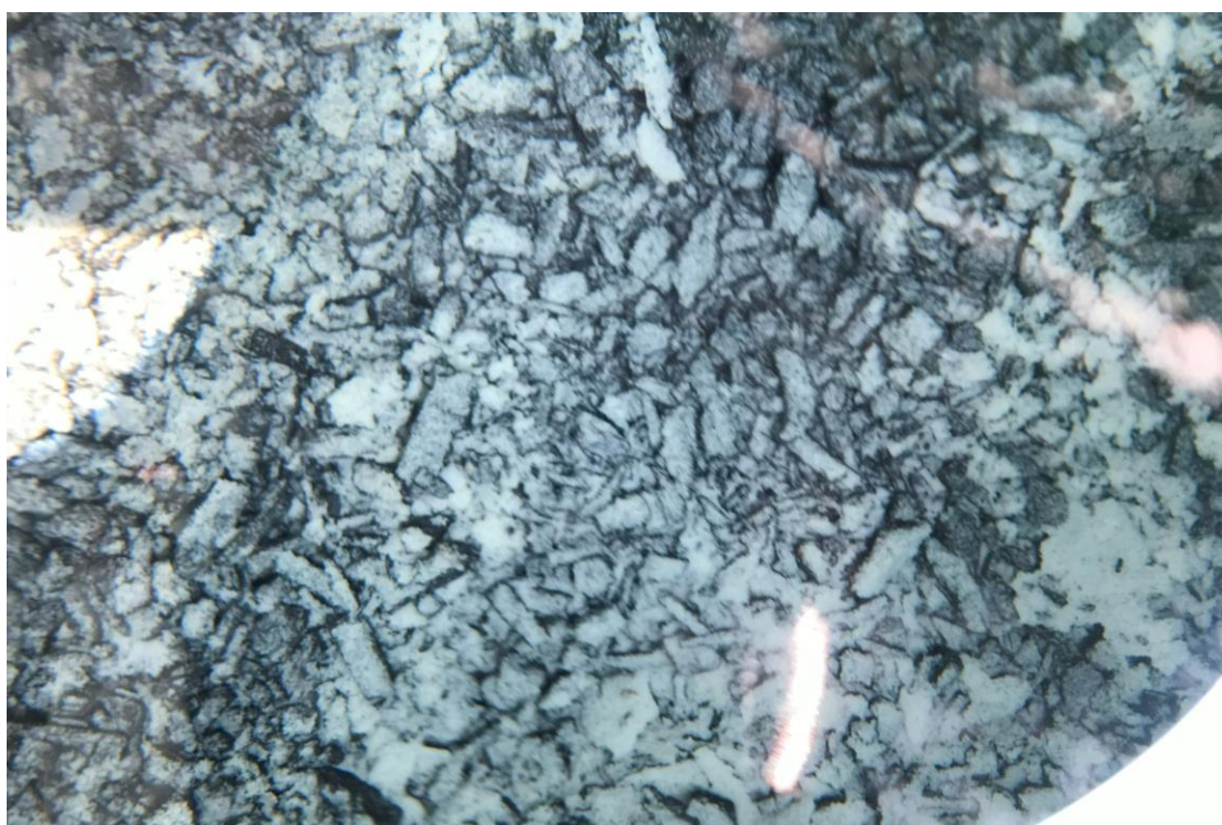
Figure 49. Surface of the biochar filter layer (possibly precipitated calcium)
