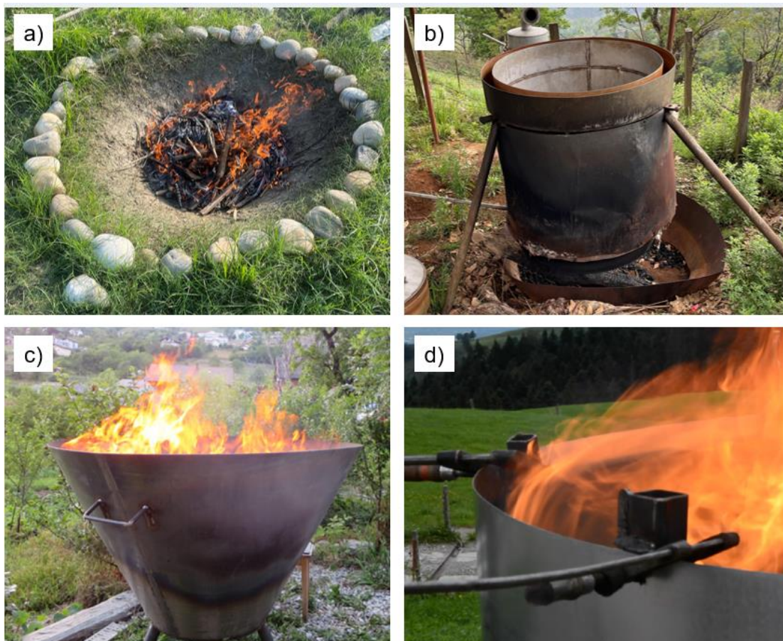
Figure 6. Different type of Kon-Tiki kilns; (a) soil-pit kiln built by us in Nepal, (b) soil-pit kiln covered by metal shield (photo taken by the author at Ithaka Insitute in Nepal), (c) deep-cone metal kiln, and (d) metal kiln with metal rim-shield.
