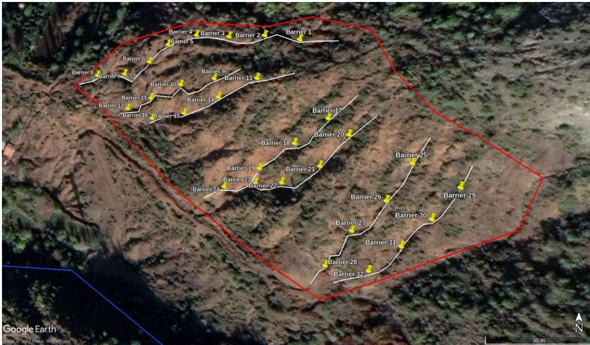
Map 4: Approximate design for area 1, with identified ravines in white and suggested location for the barriers as pinpoint.
