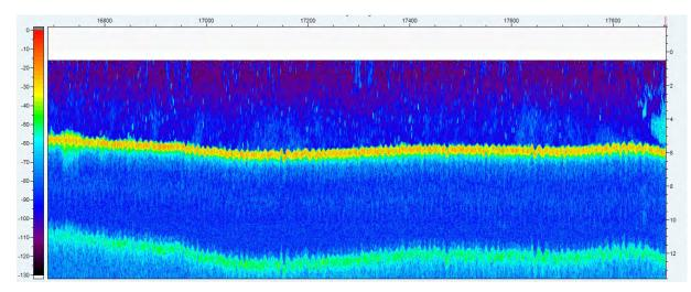
Fig. 3 — Acoustic data 30 log R echogram view on a seafloor with no seagrasses at 6m depth.
