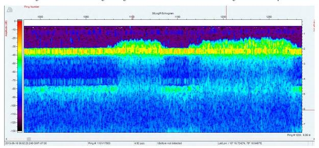
Fig. 4 — Acoustic data 30 log R echogram view on a seafloor with continuous seagrasses at 2.1m depth.
