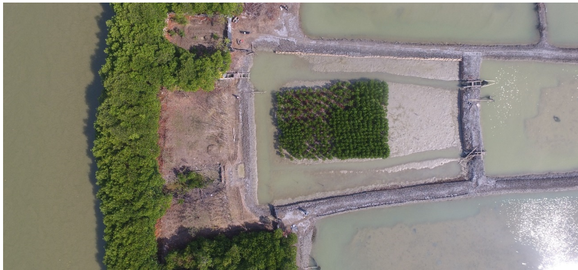
Figure 9. Each pond should have two gates, one for inflow and one for outflow, and also the mangrove section should have these two gates for optimal management of the pond water (BwNI).
