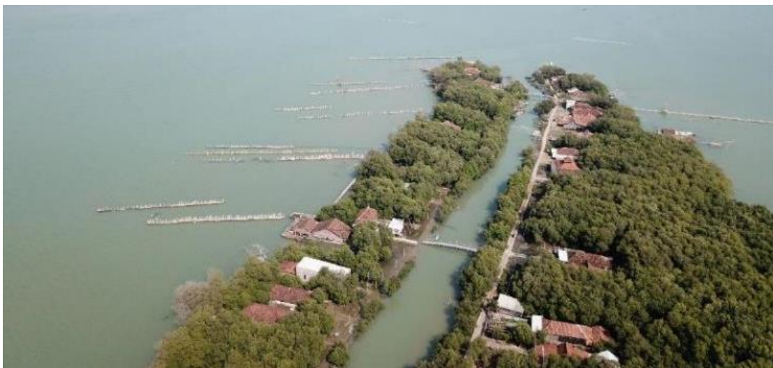
Figure 6: The villagers protect Bedono with many permeable dams (BwNI).
